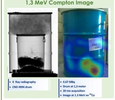
**Temporal S** is a new generation portable Compton gamma camera - spectrometer and imager - based on temporal imaging: a completely new detection concept backed by 9 proprietary patents and software.
